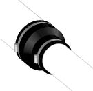
Tighten the stainless steel clamps to 60 inch-lbs. of torque.
