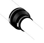
Slide the PIPECONX Coupling over the ends of the two pipes to be joined.
